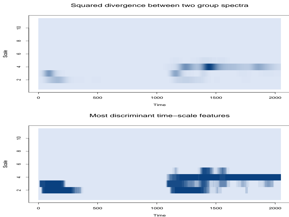
Figure 6: Earthquake vs Explosion Signals. (1, 1): Squared difference between wavelet spectra of the two groups (the darker the color, the greater the magnitude of the difference). (2, 1): Discriminant time-scale features selected (the darker the color, the larger the proportion of times the given feature was selected; p = 0.25 was used). Length of the time series is T = 2048 . Maximal scale is J = \log_2(2048) = 11 . Total number of signals in each group is N = 8 . In wavelet spectrum estimation, kernel smoothing over time was used with the Gaussian kernel and bandwidth = 100.
