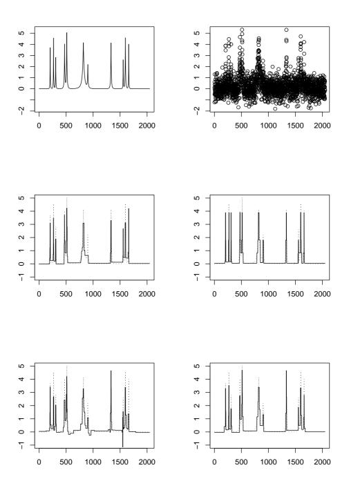
Figure 2: Top row: the bumps signal (left) and a simulated sample path (right). Middle row: reconstruction using the TS (left) and AWS methods (right). Bottom row: reconstruction using the BH (left) and UH methods (right).
