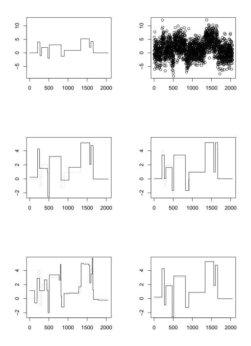
Figure 1: Top row: the blocks signal (left) and a simulated sample path (right). Middle row: reconstruction using the TS (left) and AWS methods (right). Bottom row: reconstruction using the BH (left) and UH methods (right).
